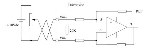
Figure 4-7 Analog AI1 Input Interface
