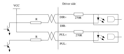
Figure 8-2 Control Terminal CN1 Signal Wiring in Position Control Mode
