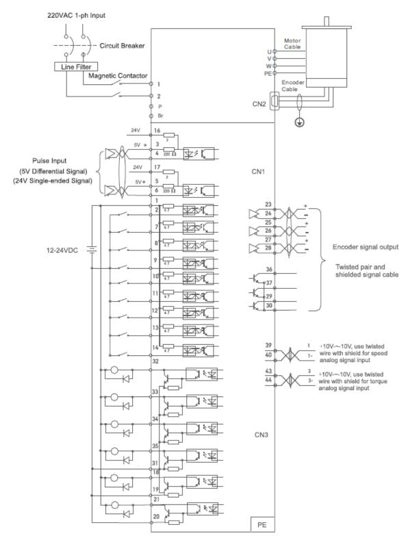
Figure 4-2 Torque/Velocity Control Mode Wiring
