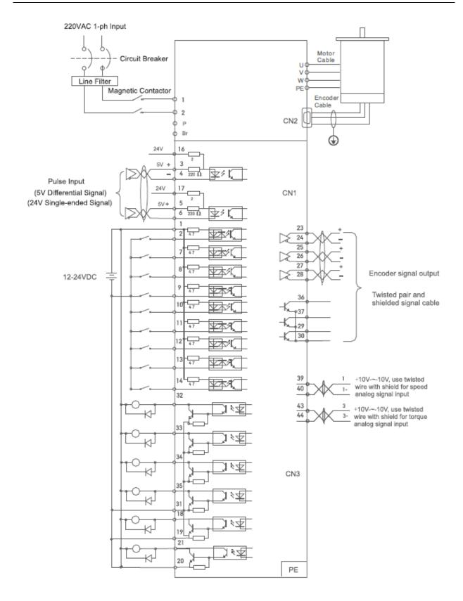
Figure 8-3 Velocity Mode Typical Wiring Diagram
