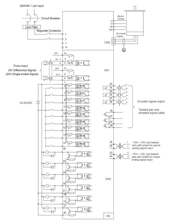
Figure 8-4 Torque Mode Typical External Wiring Diagram
