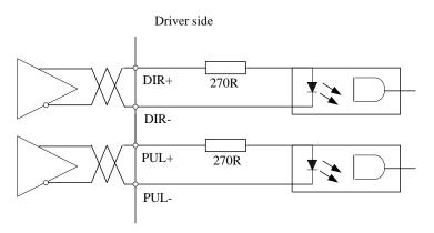
Figure 4-6 Differential 5V Pulse Signal (Pin3/Pin4/Pin5/Pin6 of CN1 Terminal)
