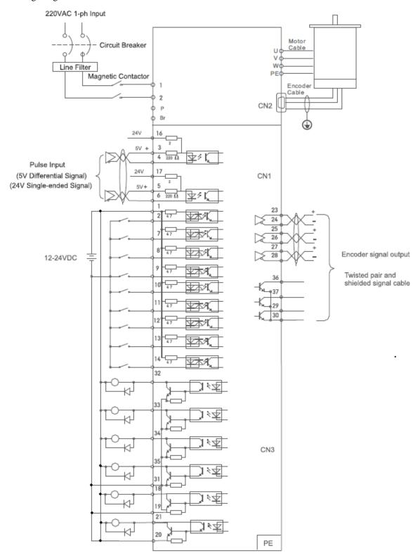
**Figure 8-1 Position Mode Typical Wiring Diagram Note:**
