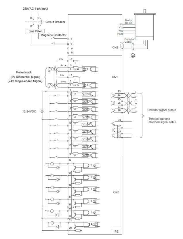
**Figure 4-1 Positional Control Mode Wiring**
