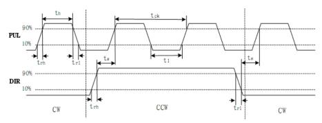
Figure 4.6 Pulse + Direction Input Interface Timing (The Maximum of Pulse Frequency: 500KHZ)
