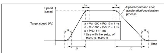
Set S-curve time for acceleration/deceleration process when the speed command is applied. According to Pr3.12 Acceleration time setup and Pr3.13 Deceleration time setup, set up sigmoid time with time width centering the inflection point of acceleration/deceleration.
