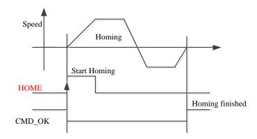
CMD\_OK and MC\_OK Both of them can be used to represent action is complete, after the signal effective, there will have a delay within 1 ms.
