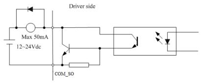
Figure 4.4 Switch Output Interface
