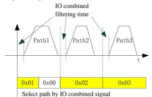
IO combined signal trigger sequence
