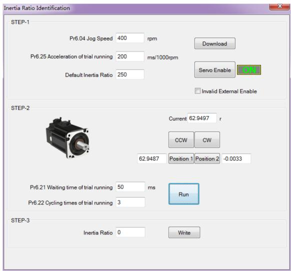
3. After finishing, Click"Write" to save the Inertia ratio identification result.
