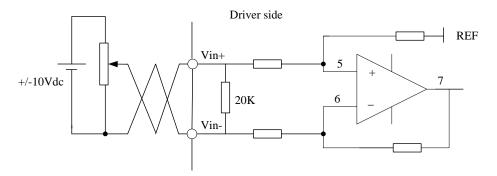
Figure 4-8 Analog AI3 Input Interface
