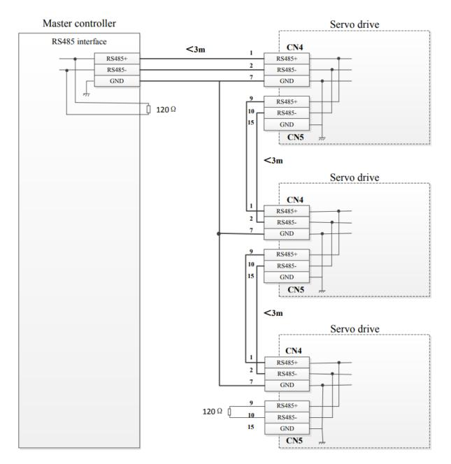
Figure: Multi-drive network connection
